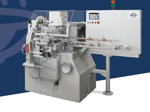
The DBD 0500-1 is the evolution of the DBD 0500 as it has now an integrated HMI to facilitate daily work. With the DBD 0500-1, Sapal offers today an upgraded single format machine with a twin wrapping head, three-side heat seal developed using the company's worldwide knowledge base and expertise and especially designed for the midrange speed wrapping of soup tablets.
